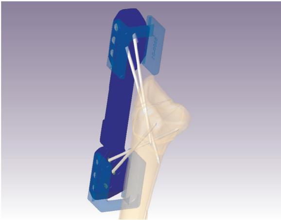
**FIGURE 8.** The spacers of the CPX device (courtesy of A.M. Surgical).
